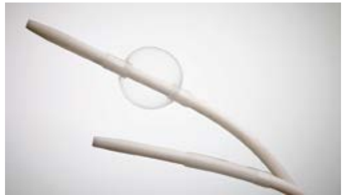
HEAT SHRINK TUBING APPLIED OVER LATEX BALLOON ENDS TO ACT AS HOSE CLAMPS AND INCREASE BOND STRENGTH
